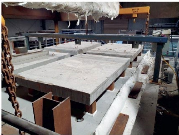
Figure 6 - Point loading of the slab whilst on the furnace
