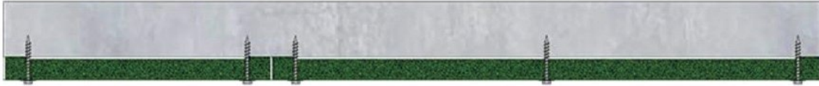
Figure 5 - Cross section / Arrangement of 120 mm thick reinforced concrete floor slab with 50mm thick TBA Firefly Intubatt fastened to the underside (exposed side).
