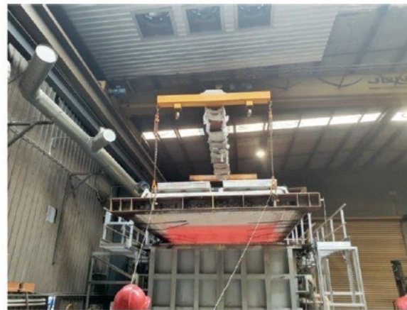
Figure 7 - View of the fire exposed side at the conclusion of the test
